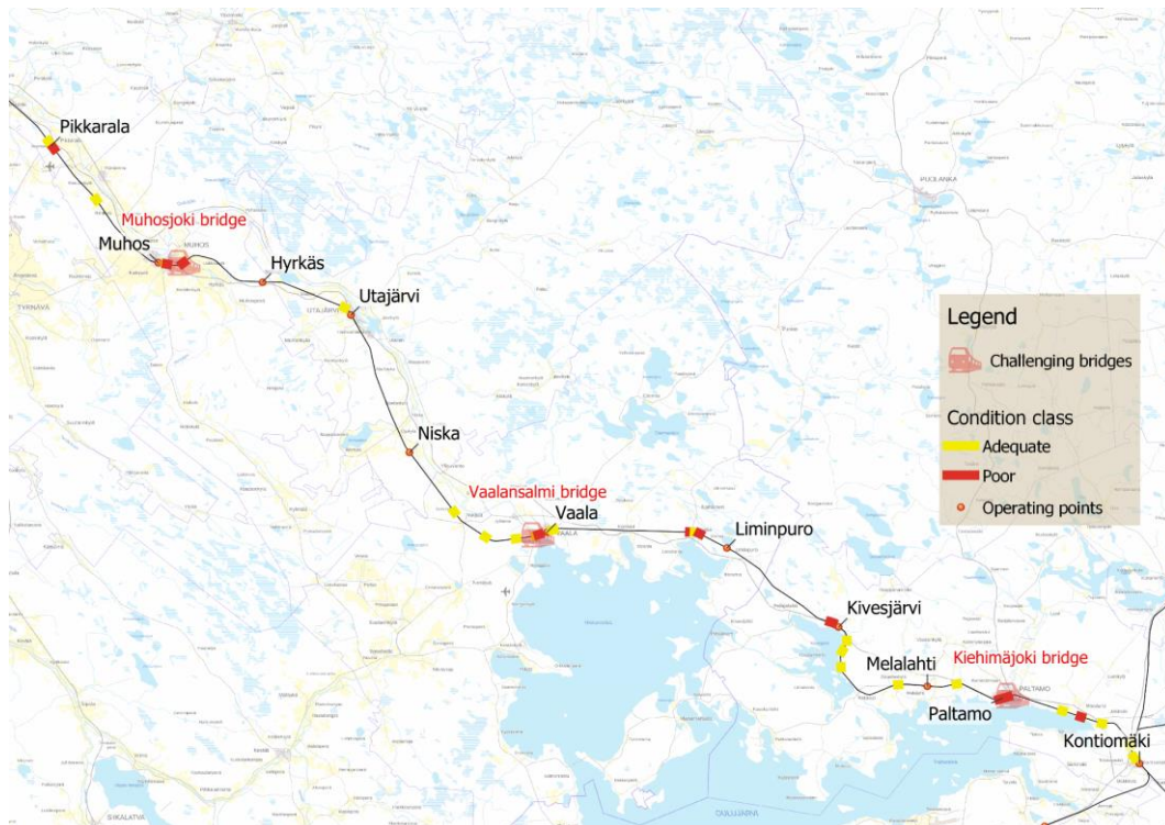
Figure 22. Track condition information. Unclassified line sections are in good condition. (Condition classification: Finnish Transport Infrastructure Agency 2020b)
